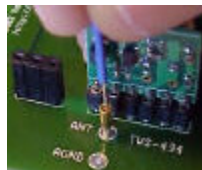
Installing 22 Gauge Wire Antenna For TWS-434
