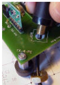
Installing Whip Antenna For TWS-434
